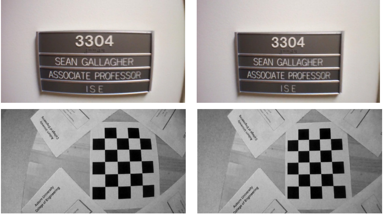
Figure 9: Distorted images (top and bottom left) and the corresponding images with distortion removed (top and bottom right)
