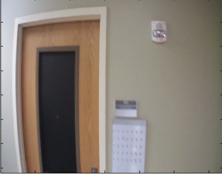
Figure 5: Image from drone camera with barrel distortion.
