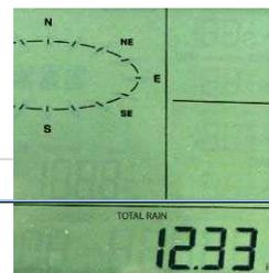
The rainfall unit can be set to read in inch or mm. The default unit is inch.
