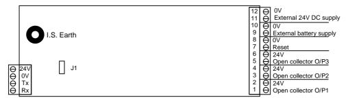
The lower 4-way connector provides a 24V and 0V connection. The voltages are always present at these terminals whilst FS2 is intact. The remaining two connections must not be used. The 24V supply is designed for use by Analox Ltd when powering external equipment. The amount of power available from this connector must be determined for each installation based upon the system configuration.
