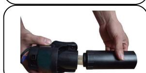
Step 2: Unscrew the black quartz sleeve cover counter clockwise and pull out quartz sleeve.
