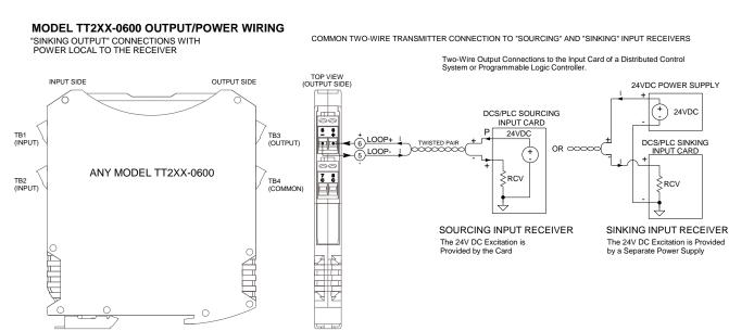
**WARNING:** For compliance to applicable safety and performance standards, the use of twisted pair output wiring is recommended. Failure to adhere to sound wiring and grounding practices as instructed may compromise safety, performance, and possibly damage the transmitter.
