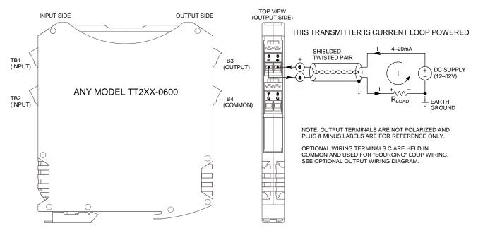
The traditional loop-powered "sinking" output connections are shown above. Shielded twisted-pair wiring is often used at the output to connect the longest distance between the field transmitter and the remote receiver as shown. The output of this transmitter fluctuates relative to earth ground by the voltage drop in the load and connection wire. This makes it flexible in the way it connects to various "Receiver" devices.
