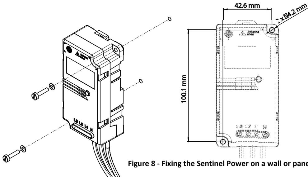
Figure 8 - Fixing the Sentinel Power on a wall or panel
