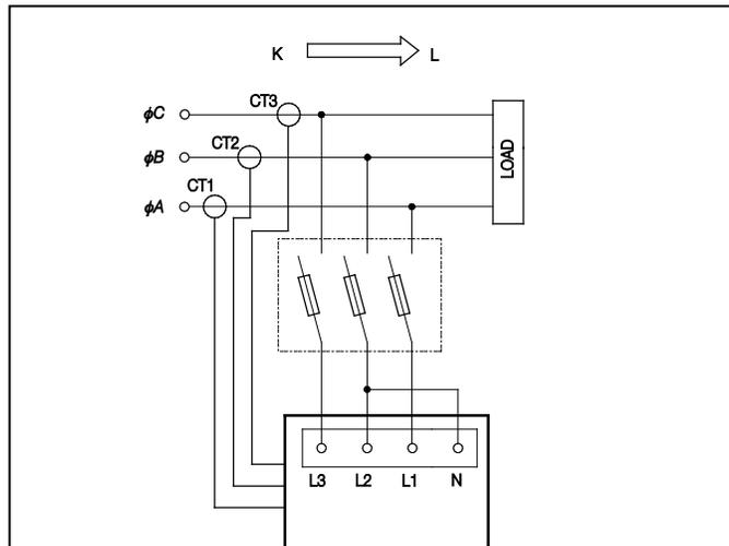
Figure 11 - Example of Fuse holder connection
