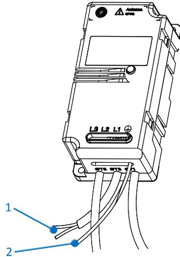
**Figure 13 - Connecting the wires to the Input Voltage**
