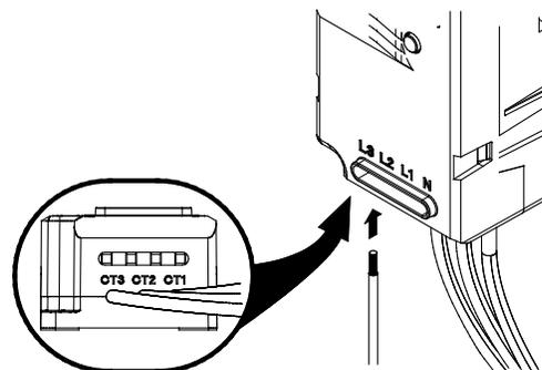
Figure 12 - Connecting the wires to the Input Voltage
