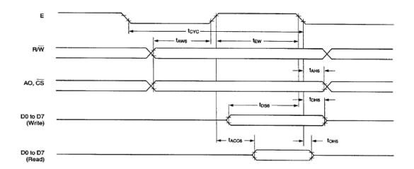
Note: toyos indicates the interval during which CS is LOW and E is HIGH.
