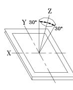
Inspection should be performed within  $\emptyset$  ( $\emptyset$ =30°) from Z axis to each X and Y axis.
