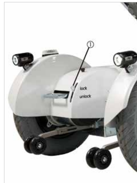
Fig. 42: Brake release lever (emergency release)
