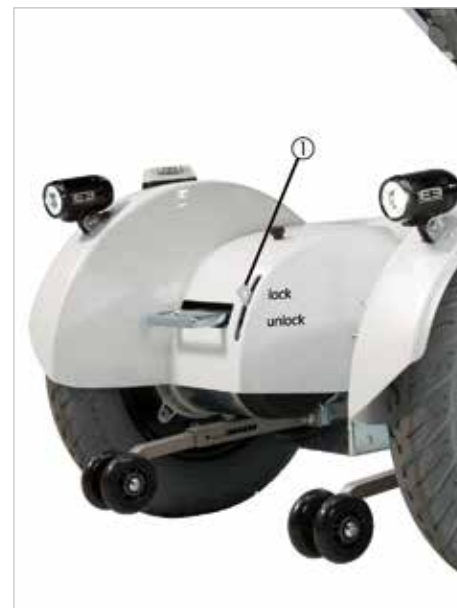
Fig. 38: Brake release lever (emergency release)
