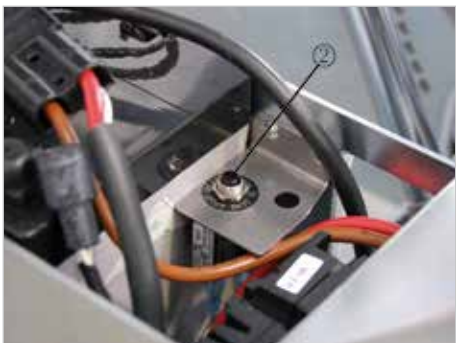
Fig. 80: Secondary safety switch
