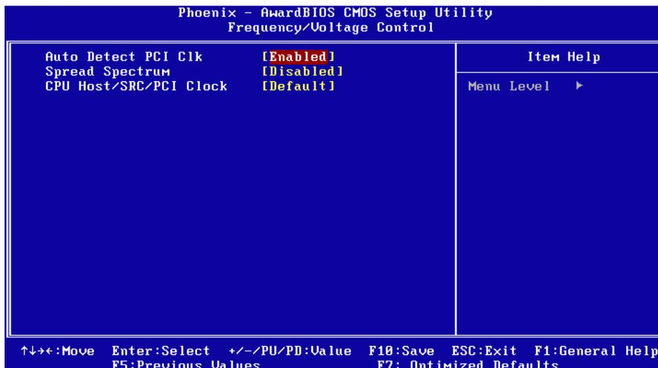
**Note!** This “Frequency/Voltage Control” option controls the CPU Host and PCI frequency, this page is developed by CPU and Chipset independent, some items will show up when you install a processor which supports this function.
