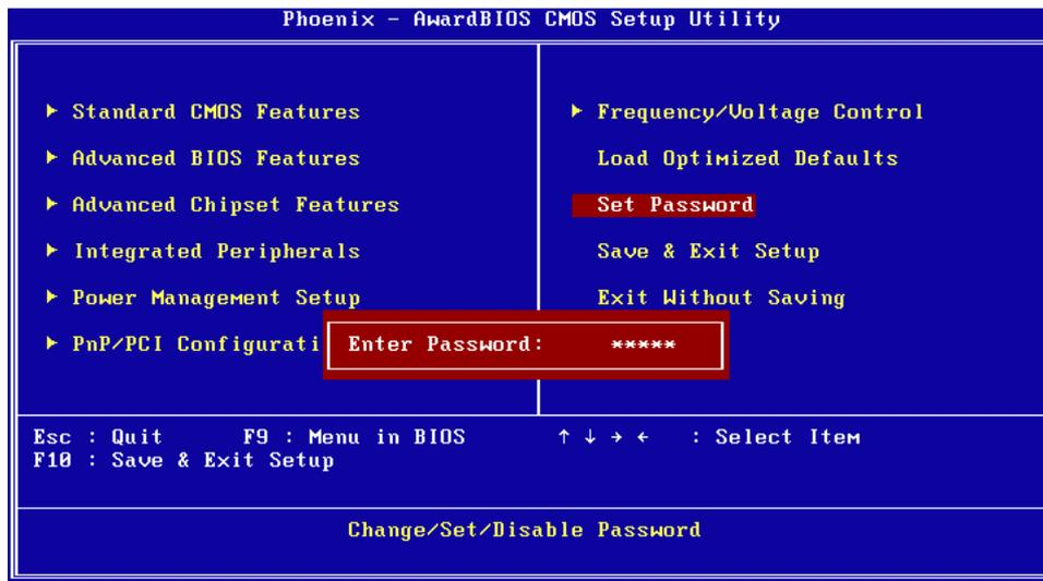
**Note!** *To enable this feature, you should first go to the Advanced BIOS Features menu, choose the Security Option, and select either Setup or System, depending on which aspect you want password protected. Setup requires a password only to enter Setup. System requires the password either to enter Setup or to boot the system. A password may be at most 8 characters long.*
