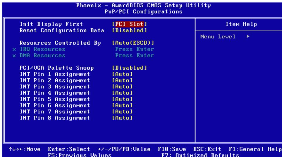
**Note!** This “PnP/PCI Configurations” option is setting up the IRQ and DMA (both PnP and PCI bus assignments).
