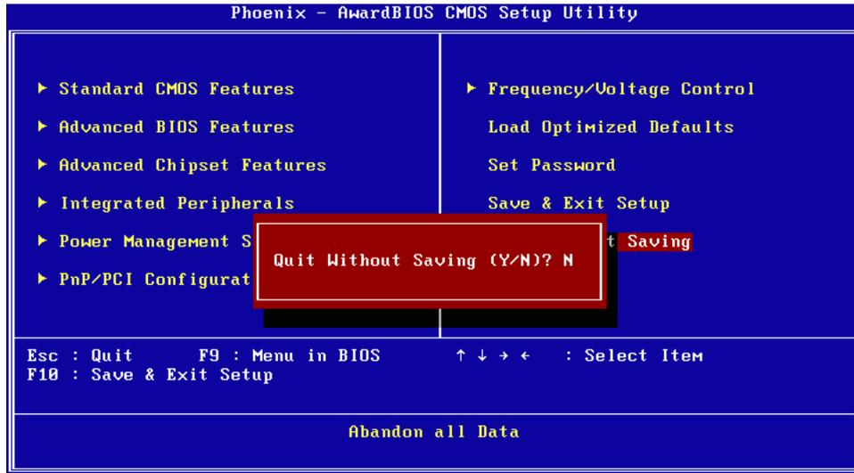
**Note!** Typing “Y” will quit the BIOS Setup Utility without saving to CMOS. Type “N” will return to BIOS Setup Utility.
