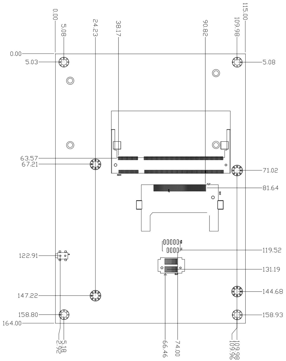
**Figure 2.4 PCM-4372 Dimension BOTTOM**
