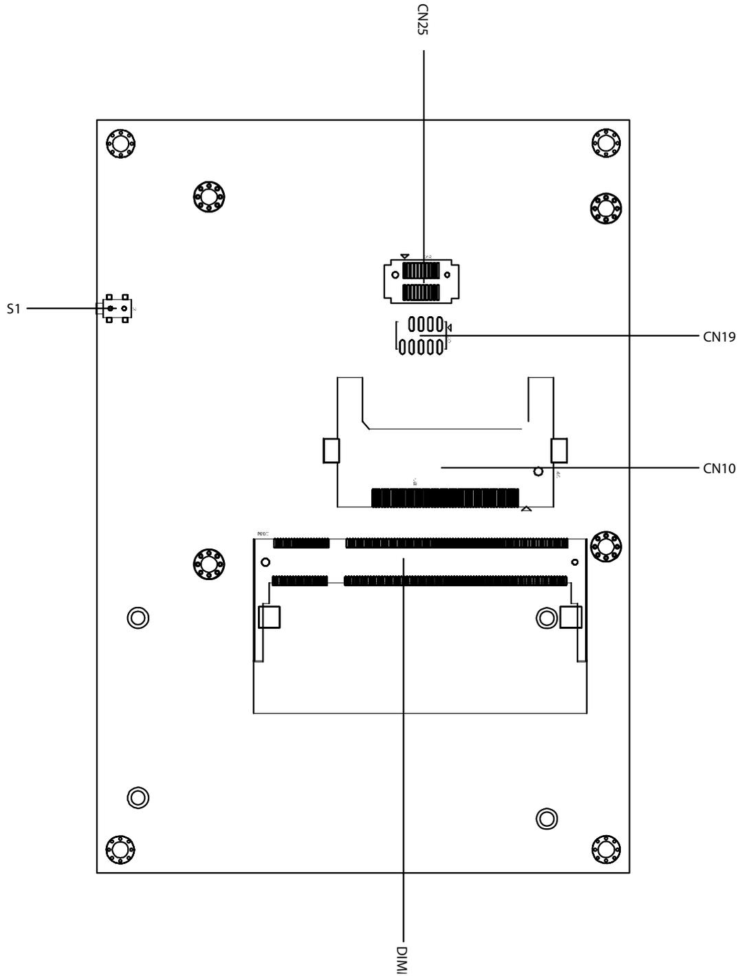
**Figure 2.2 PCM-4372 Position BOTTOM**
