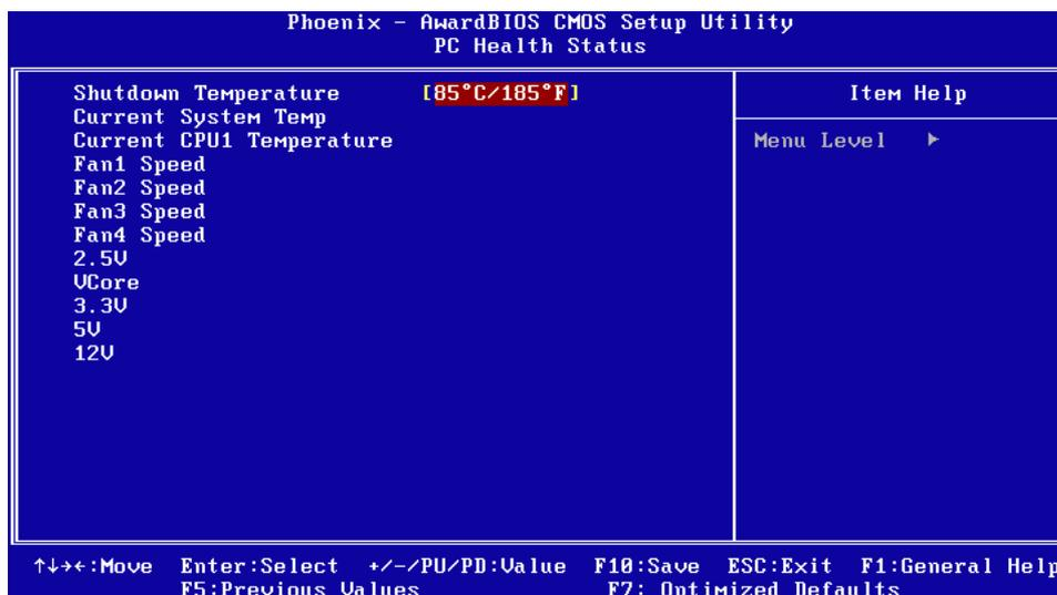
**Note!** This "PC Health Status" option controls the Thermal, FAN and Voltage status of the board. this page is developed by Chipset independent.
