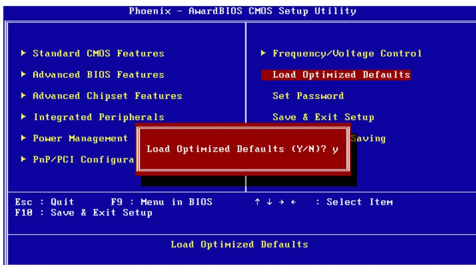
**Note!** *Load Optimized Defaults loads the default system values directly from ROM. If the stored record created by the Setup program should ever become corrupted (and therefore unusable).*
