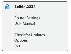
The Belkin Router Manager appears in your system tray (Windows) or menu bar (Mac). Its icon indicates the current status of your Router and also allows you to access your Router's settings to make changes. It also provides quick access to software that came bundled with your Router.
