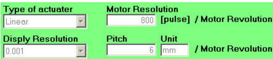
Encoder resolution unit and axis mechanical data are read from the connected axis, therefore this menu
