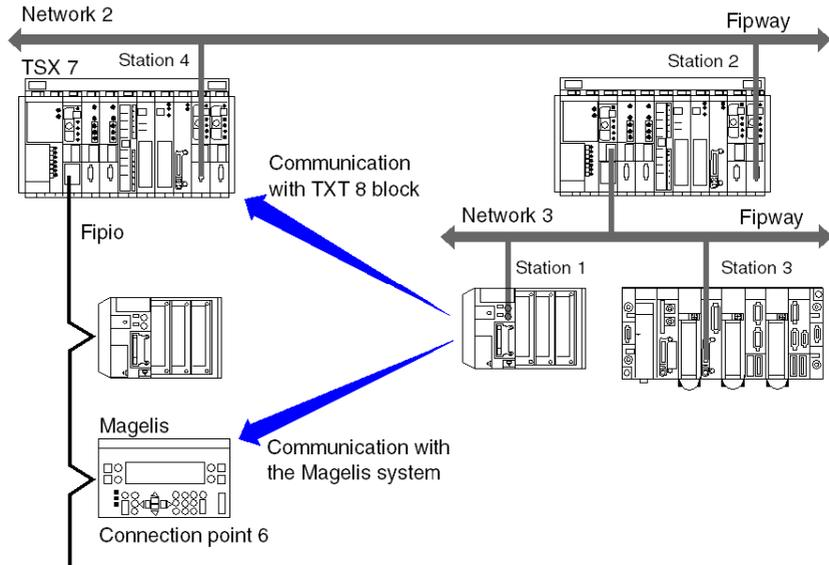
The address of the TXT 8 text block on the TSX 7 PLC station 4 is:
