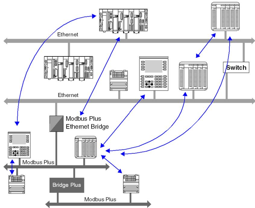
**NOTE:** Access is possible from devices on the Modbus Plus network across Ethernet/Modbus Plus bridges. In contrast, the devices on the second Modbus Plus network cannot be accessed by an Ethernet device via the Bridge Plus.
