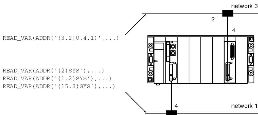
All messages intended for network 3 are sent to the coupler with module address 4, and those whose destination network is 1 to the network link integrated into the processor.
