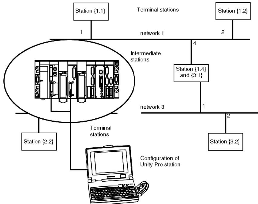
**NOTE:** Multi-network routing information is constructed at the station level at the time of configuration of each bridge. No consistency check is done on routing data for the same network architecture.
