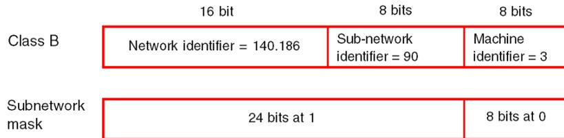
The segmentation allows for 254 possible sub-networks with 254 sub-network machines.
