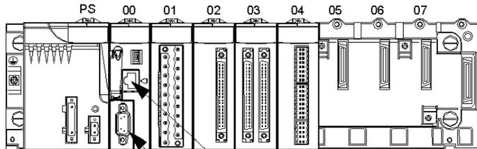
Rack 0, Module 0, Channel 3: Ethernet port
