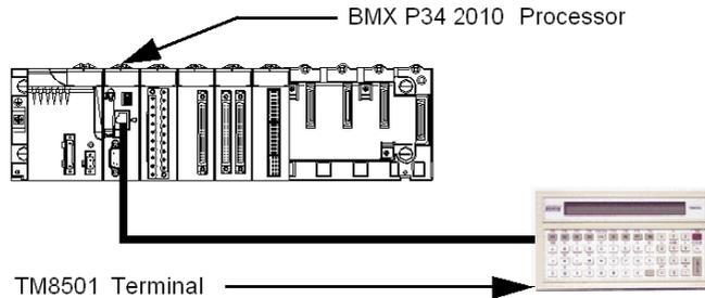
The address settings of the TM8501 terminal are `ADDM ('0.0.0')` or `ADDM ('0.0.0.SYS')`.
