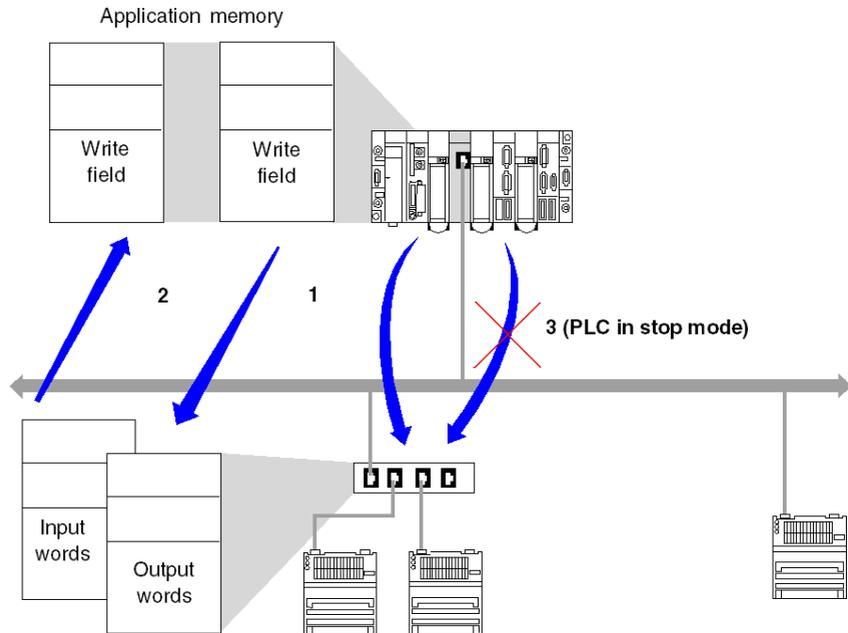
1. As soon as the PLC goes into Run mode, the module opens one connection per scanned device.
