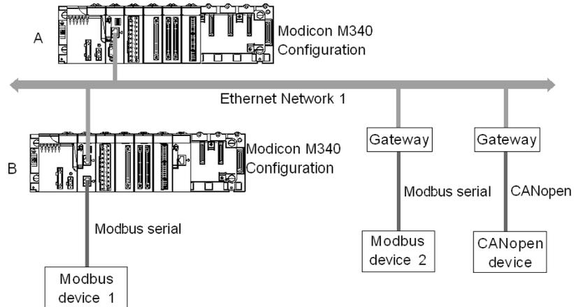
In the diagram above there are two Modicon M340 configurations which are called A and B. The configuration B is directly connected to the Modbus device 1 via Modbus communication channel.
