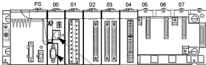
Rack 0, Module 0, Channel 0: Serial port
