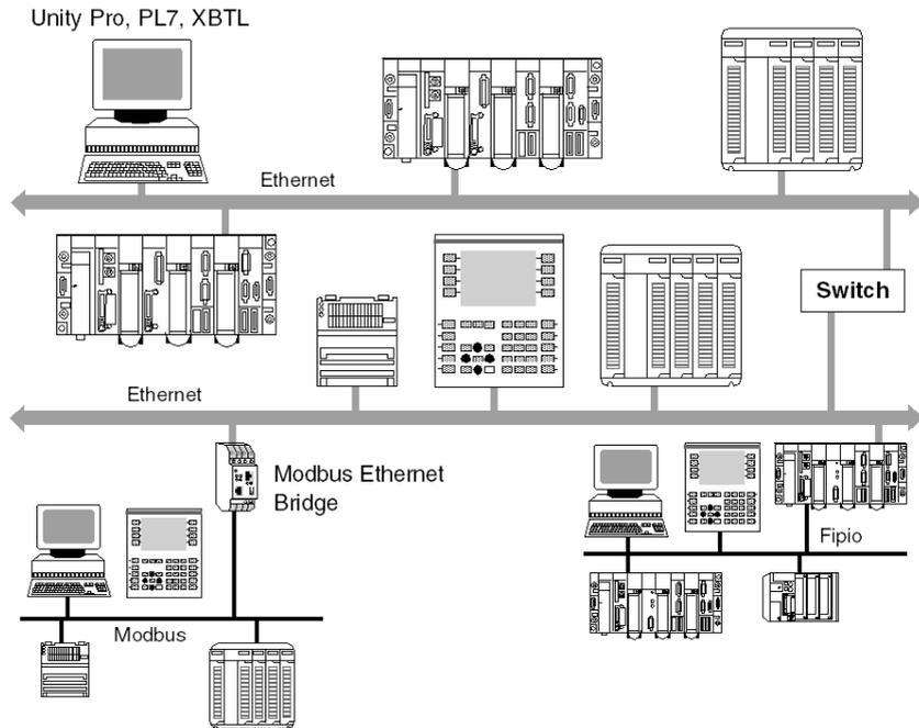
**NOTE:** Depending on the type of network used, the interconnection is made either directly via a PLC which routes the information (Ethernet/Uni-Telway), or via an additional device such as a bridge (Ethernet/Modbus) or switch (Ethernet/Ethernet).
