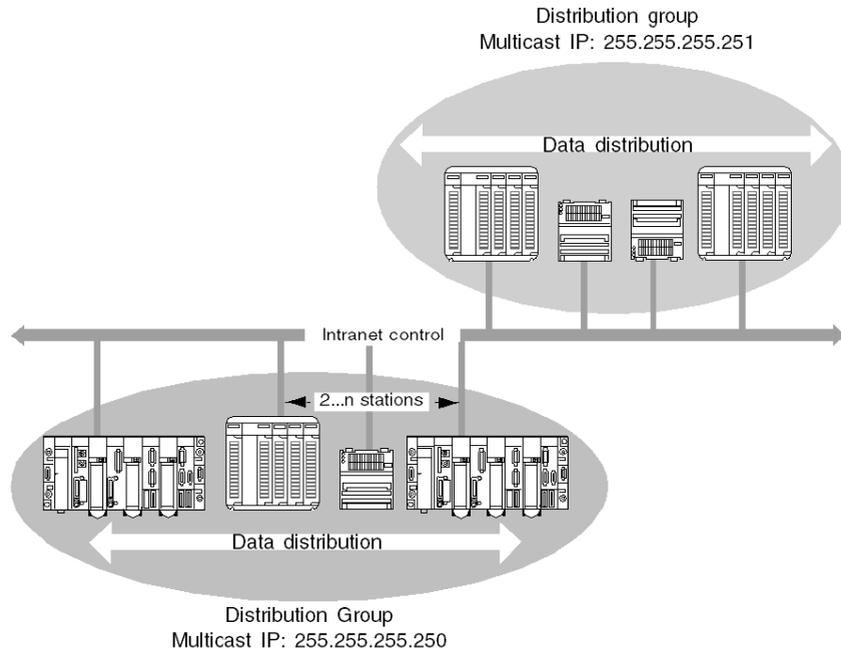
A **Distribution group** is a group of communication modules identified by the same **multicast IP** address. Exchanges in "multicasting" are used to distribute **Global Data**. Several independent distribution groups can co-exist on the same subnetwork with their own multicast address.
