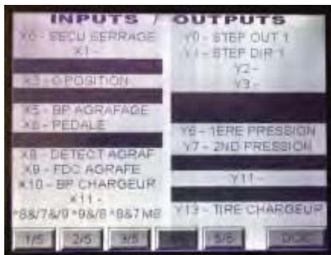
Page 4 enables visualisation of Input/Output. This page is functional, even during continuous operation of the machine.
