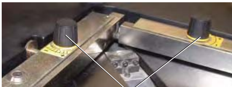
( RI ) BUTTONS FOR ADJUSTING STOP ANGLES
