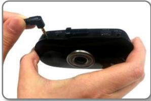
Connect External GPS to GPS connection on V200HD body.
