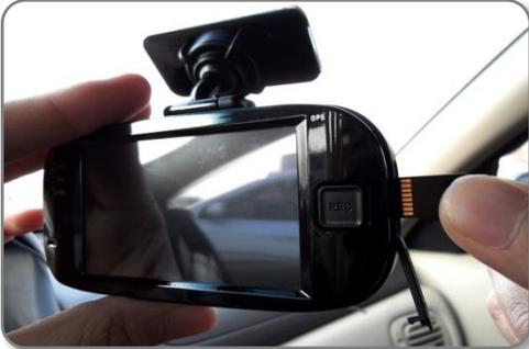
Insert Micro SD card to V200HD SD card slot.
