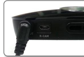
Connect a TV-Out cable to the TV-Out jack on a V200HD body.
