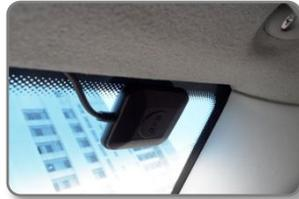
Attach GPS module at well visual place and tidy up a cable.
