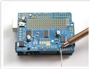
Solder each one of the pins into the shield to make a secure connection
