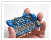
Finally, break off a 2-pin piece of header and place it next to the POWER terminal block, short legs down, tape it in place if necessary and solder it in.
