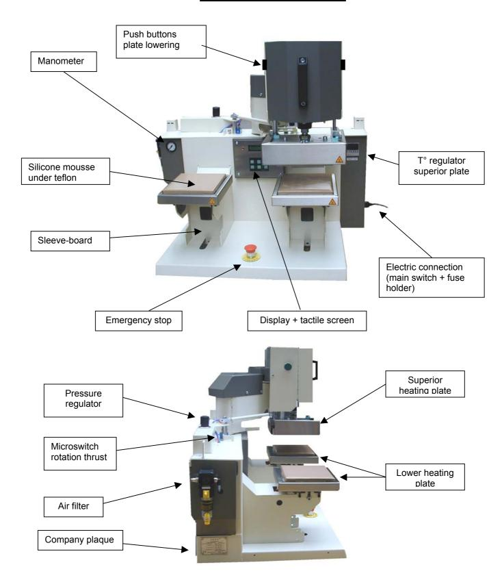
This heat seal press is standard to the article L 233-5 of the labour laws, to ensure the safety of the user.
