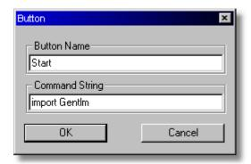
The Command Button dialog lets you specify the button name, that is that text that is display on the button, as well as the command string to be executed. Upon execution a new CMDSTRING block will be generated with the contents of this command string copied into the CMDSTRING block. Then the CMDSTRING block is processed by the GSEOS command processor and forwarded to the Python interpreter.
