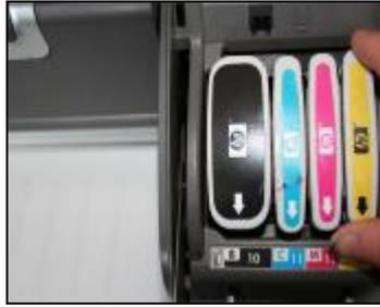
Remove out the original cartridges
