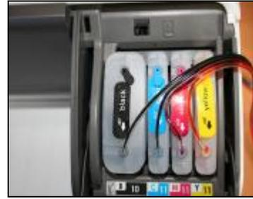
Place the cartridges of our CISS correctly
