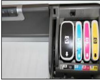
Open the cover for the cartridges
