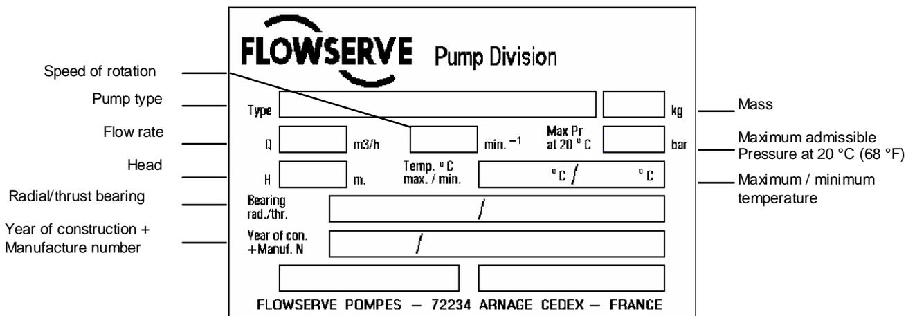
Each pump unit is supplied with the following nameplate:
