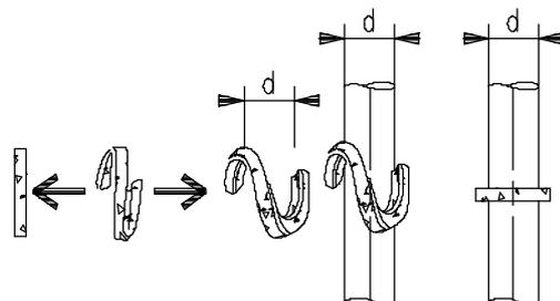
After setting the last packing, fix the gland on the packing and screw up the nut by hand.
