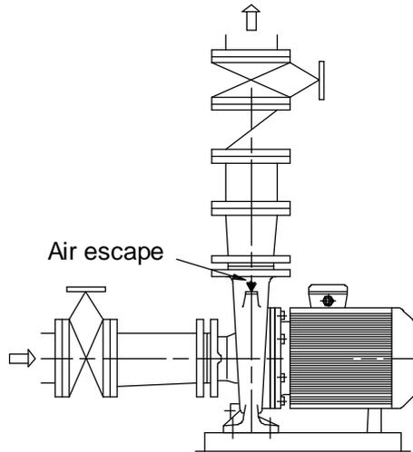
**Priming of a flooded pump**
