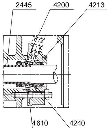
**!** **CAUTION** With a mechanical seal, the maximum temperature is limited to 80 °C (176 °F) whatever the internal construction of the pump is (Cast iron or Bronze).
