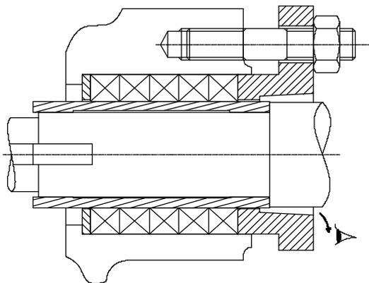
**!** Shield grids being removed during installation of the gland packing, it must be ensured that they are replaced as soon as this operation is completed.
