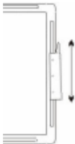
Mounting bracket slides to any position.
