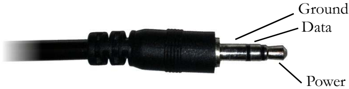
Figure 1: 3.5mm Stereo Plug Wiring
