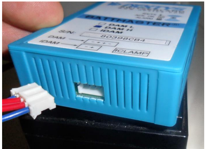
Figure 16: Cable connection to the DAM
