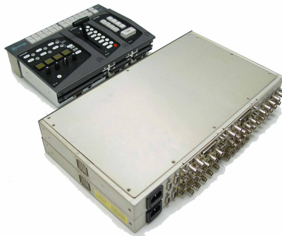
Figure 1-1 The iris system with all options fitted requires two 1RU chassis
