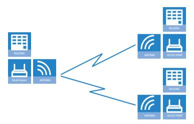
When using Access Points and appropriately polarized antennas in accordance with IEEE 802.11n two wireless links ("spatial streams") can be established simultaneously between the end points of a point-to-point connection. This allows higher data throughput to be achieved or greater distances to be covered than when using other standards.
