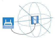
To simplify the problems of representing three-dimensional power distribution, two planes (horizontal and vertical) are taken and the emitted power is plotted as measured in various directions.
