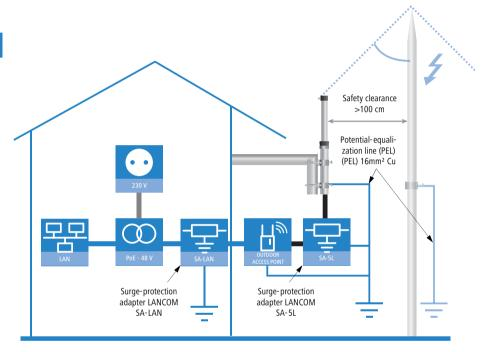
In this case, the AirLancer Extender SA-5L surge-protection adapter is installed directly between Access Point and antenna and grounded for example via the antenna's potential equalization line.
