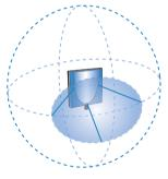
The power fed into the antenna is focused, and thus amplified, into a main beam direction. This amplification is referred to as "gain". The greater the focusing, the greater is the antenna gain.
