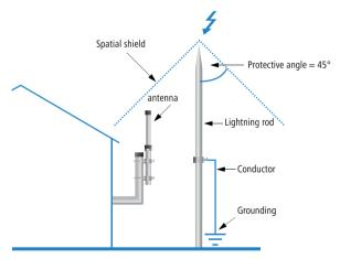
Distance of the lightning rods from the antenna: Positioning the lightning rod a sufficient distance away from the antenna prevents the conducted lightning charge from flashing over to the antenna or other conductive components. This distance can be calculated exactly on the basis of several factors. However, in practice a safety clearance of more than 100 cm is generally sufficient.
