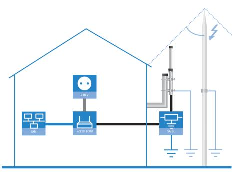
The central component for internal lightning protection is the AirLancer Extender SA-5L surge adapter. The employment of the AirLancer Extender SA-5L is **essential under all circumstances**—despite outer lightning-protection measures, partial discharges can still give rise to surges that can damage sensitive WLAN modules.
