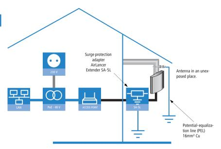
The basic situation shows an application where the antenna is not mounted in an exposed place — there is therefore no danger of a direct lightning strike.
