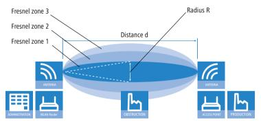
The Fresnel zone 1 must remain free from obstruction in order to ensure that the maximum level of output from the transmitting antenna reaches the receiving antenna. Any obstructing element protruding into this zone will significantly impair the effective signal power. The object not only screens off a portion of the Fresnel zone, but the resulting reflections also lead to a significant reduction in signal reception.
