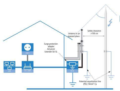
In this example the antenna is mounted in such a way that a direct lightning strike is possible. A lightning rod with a sufficiently large safety clearance of more than 100 cm is installed as a protective measure.
