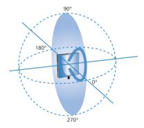
The bold line indicates the power that was measured in a certain direction. If this line reaches the outer limit of the "ideal radiation sphere", then the maximum antenna power is radiated in this direction. The closer the bold line
