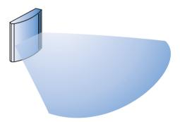
■ Directional antennas have beams with narrow horizontal and vertical angles, for example of 9°. Directional antennas are mainly used on rooftops or masts for establishing point-to-point links that interconnect areas of a network that are separated by a distance.
