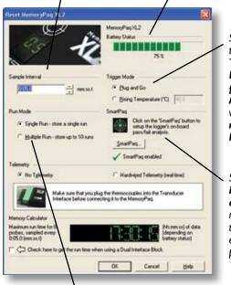
Set data-recording to start when Transducer Interface is plugged into MemoryPaq, or when temperature rises to a given level.
