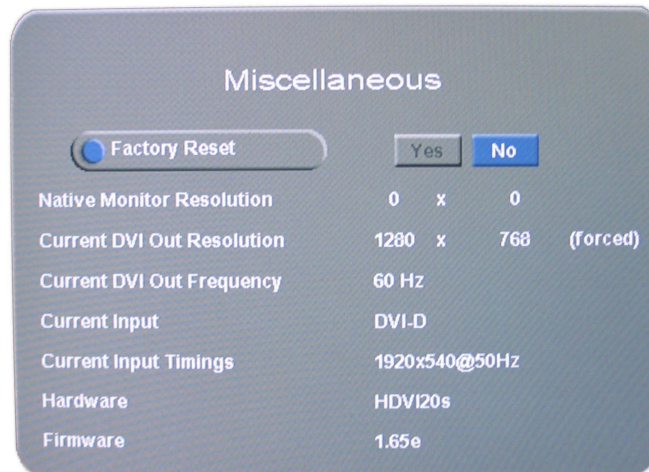
Figure 15: “Miscellaneous” Window Example
