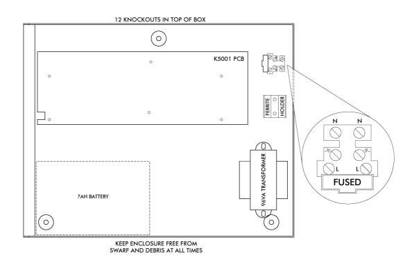
Annex 2. – Field wiring and PCB connector details.
