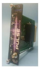
The PULSE '2070' plugs directly into a 2070 Controller, which provides power and serial data through the edge connector. Data from your serial device is transparently sent to other ENCOM PULSE Wireless Modems using license free 900 MHz technology. LED indicators on the front panel provide serial and RF status information.
