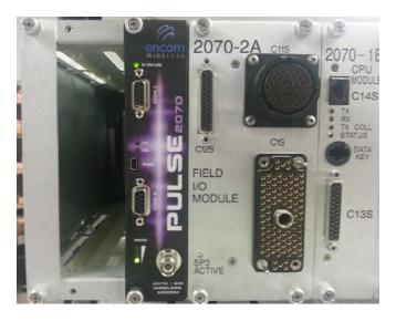
The Controller can be powered ON when the PULSE Modem is plugged in. Site specific regulations and/or practices may not allow equipment to be connected or disconnected when power is applied. If these regulations are in effect, ensure the 2070 Controller is powered down prior to installation.
