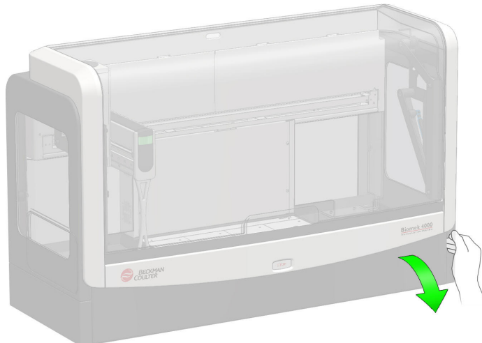
Figure 22 Integration Deck Door—Opening
