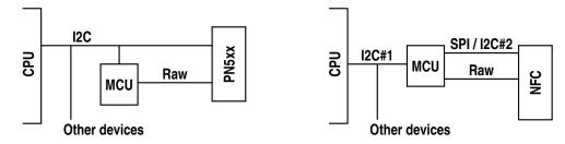
Sharing the same bus for communication between all three parties would allow operating the NFC chip from the CPU without involving the MCU at all. As a drawback, the MCU would have to switch between master and slave roles, and communication between MCU and NFC chip would increase occupancy of the  $I^2C$  bus and be subject to its arbitration rules.
