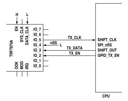
Furthermore, the interface must remain selected. If the SPI bus is shared with other devices, it must therefore be held until the send or receive operation – or sequence of operations – is complete.
