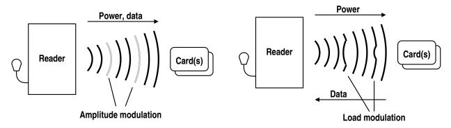
The reader sends data to the card (drawing on the left) by modulating the field it emits. It typically uses some form of Amplitude Modulation (AM), though other modulation schemes are possible. The card sends data to the reader (drawing on the right) by changing the characteristics of its receiver and thus modulating the field created by the reader. This is called load modulation.
