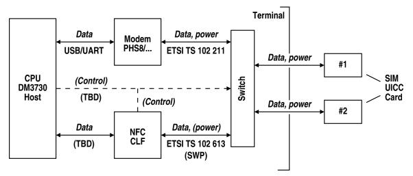
Modem and NFC subsystem both access the SIM cards through a switch that distributes data signals and power from both sources to the cards. The modem communicates with the protocol defined in [22], while the NFC subsystem uses the Single Wire Protocol (SWP) defined in [23]. Both protocols share the same power rails but use different signals for communication.
