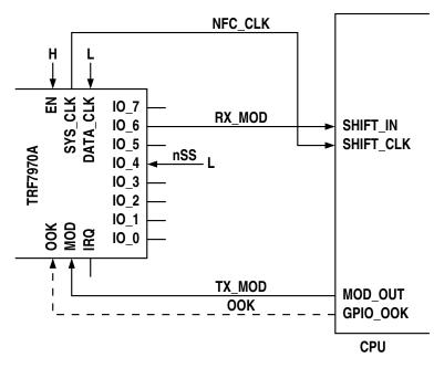
The OOK control signal allows the host to change "on the fly" between OOK or Amplitude-Shift Keying (ASK). It is presently not clear under what circumstances such functionality would be required.
