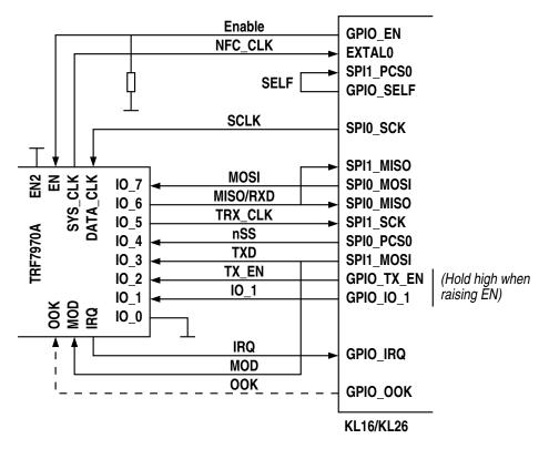
Note that no external switches or multiplexers are required. As explained in section 3.1 of [50], inputs that are driven high while the chip is not enabled draw a significant idle current. To avoid this, IO\_1 should be connected to a GPIO and only be driven high when needed for interface selection, and the SPI bus should not be shared with other devices.
