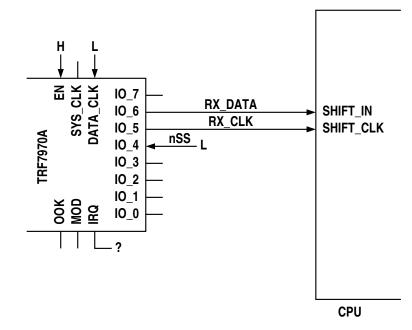
As in SDM, nSS has to be held low while using either DM0 or DM1. The documentation is inconsistent as to whether interrupts may be generated in DM1.
