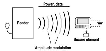
Communication is exactly the same as with a card: the reader modulates the field to send data to the phone, and the phone modulates the field by changing its load characteristics to respond.
