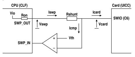
In this circuit, the comparator would output a "1" if
