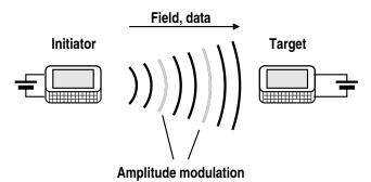
Communication between initiator and target can be as if they were reader and card, respectively, with the initiator providing the field and the target modulating it. The main difference is that the target has its own power supply and thus does not depend on the presence of an initiator to operate.
