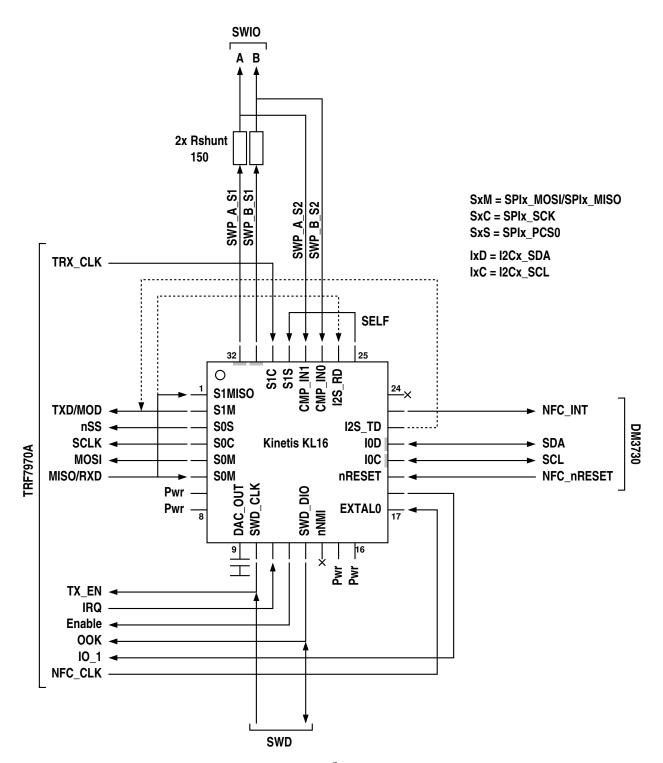
The dotted lines indicate connections for using  $I^2S$  instead of SPI for raw modes. If the pins are not used for anything else, the circuit can connect to both sets of pins, thus leaving the choice of communication mechanism to the firmware.
