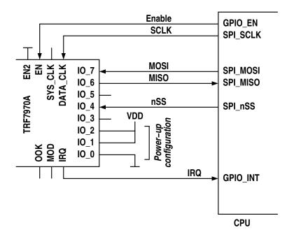
The transceiver operates as a SPI slave and the SPI bus can be shared with other devices.
