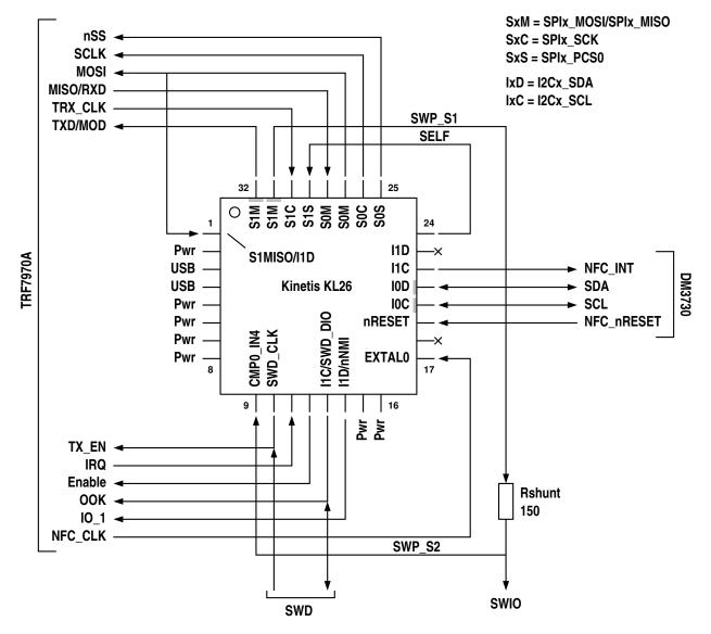
The pin descriptions only list functions pertinent to a possible use in Neo900. The KL26 makes extensive use of multiplexing and most pins have between four and six different functions.
