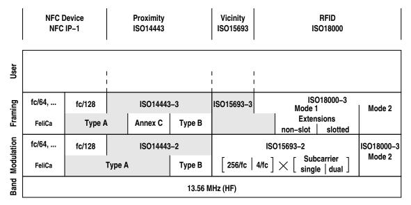
Where protocols are shared across families, the origin of the protocol is shown with a grey background. For example, ISO 18000-3 Mode 1 without extensions uses the anti-collision protocol defined in ISO 15693-3. Proprietary protocol variants like MIFARE<sup>TM</sup> or FeliCa<sup>TM</sup> are not shown.
