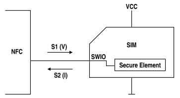
The lower layers of SWP are defined in [23]. It is intended to convey configuration data and radio messages related to ISO 14443-3 type A [7] and NFC IP-1 [3] between NFC and the Secure Element in the SIM.
