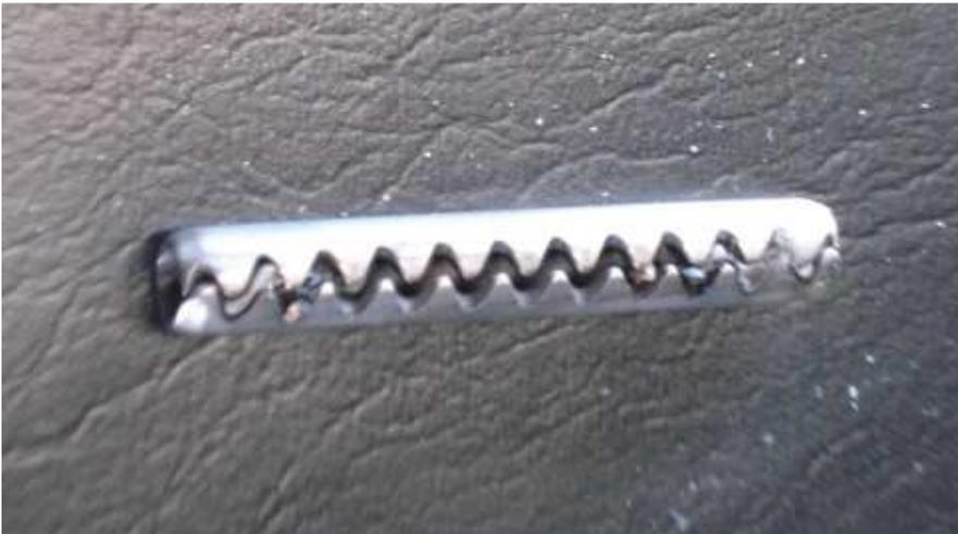
Step 3) Tap the Company23 roll pin tool to install the new axle pin. The pin should be installed flush with the CV axle's outside diameter. Twist the tool as you remove it.
