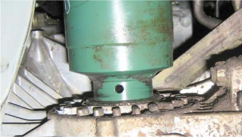
Step 2) Insert the Company23 axle pin tool's small end into the inside of the new roll pin.
