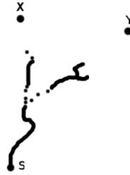
Figure 2.1: Pask’s experiment. S, X and Y are electrodes located on a plane immersed in a solution of metallic ions. Voltage is applied to the electrodes to create a potential between S and X, and between S and Y.
