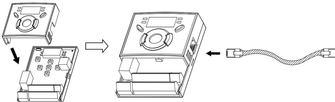
3) Connect the other side of the remote cable to the remote keypad as shown below.
