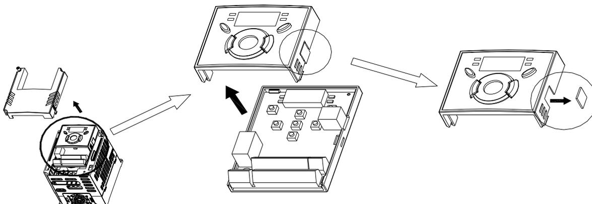
2) Attach the top cover of the I/O board kit and connect the remote cable as shown below.
