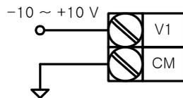
When using -10 ~ 10V from external circuit
