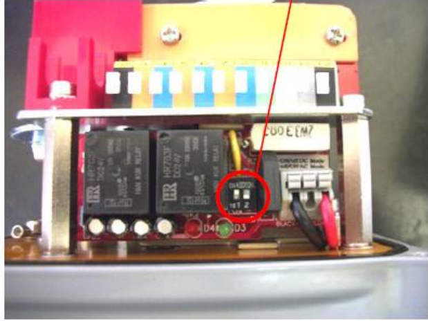
DC OPERATION DIP SWITCH 1 UP - DIP SWITCH 2 DOWN
