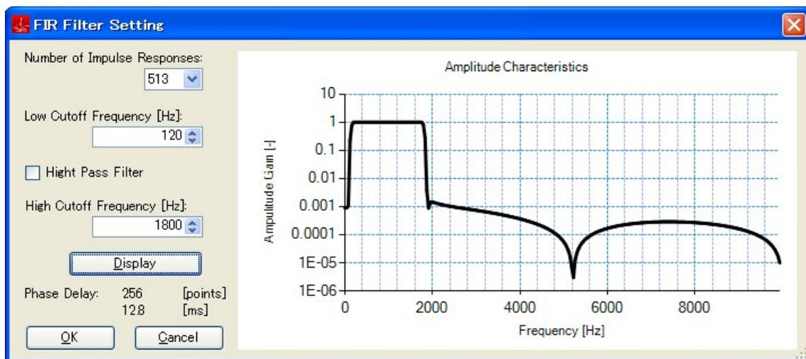
[FIR Filter Setting] Dialog (after setting parameters)
