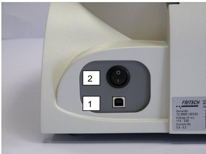
The laser is switched on and off with the on/off switch (2).
