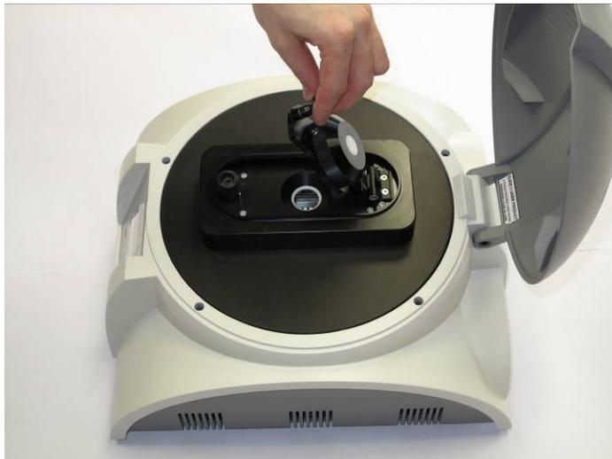
4. Seal the measuring cell lid by pressing down firmly on the button (1) and turning the locking screw (2) clockwise at the same time.
