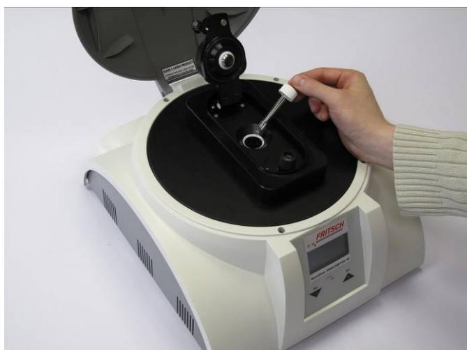
2. Turn the rotary knob (1) to the position "up" before closing the measuring cell lid. This ensures that the glass rod that forms the top part of the measuring cell is oriented upward.
