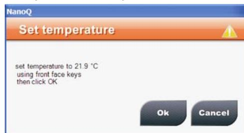
4. When the temperature shown in the display of the ANALYSETTE 12 DynaSizer has reached the configured measuring cell temperature, click on "OK".
