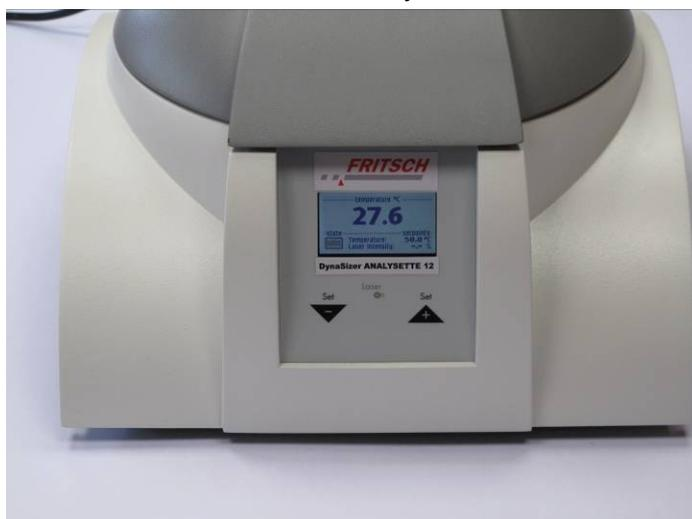
The stability of the sample temperature is shown in the field on the lower left:
