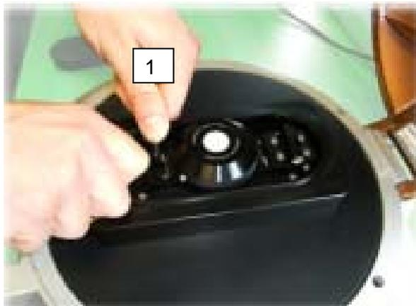
3. Open the measuring cell to make certain that it is completely free of residual dust or liquids.
