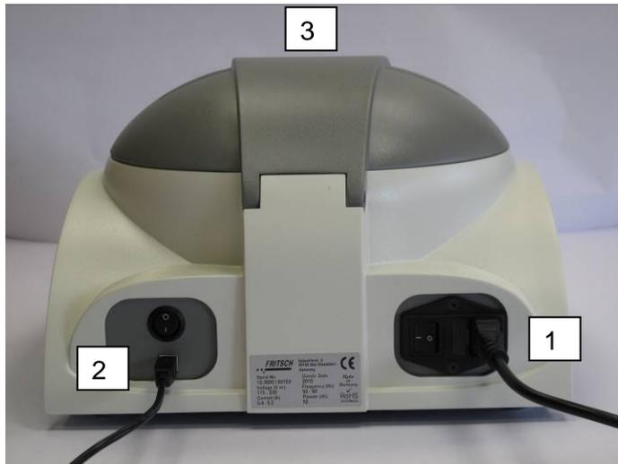
2. Switch on the instrument with the main switch (4) on the back by setting the main switch to the position "I".
