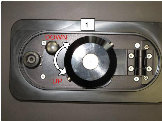
3. Fold down the measuring cell lid to close the measuring cell.
