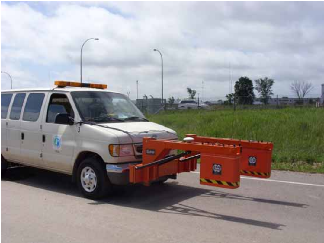
Figure 2.2 New GPR vehicle antenna mount
