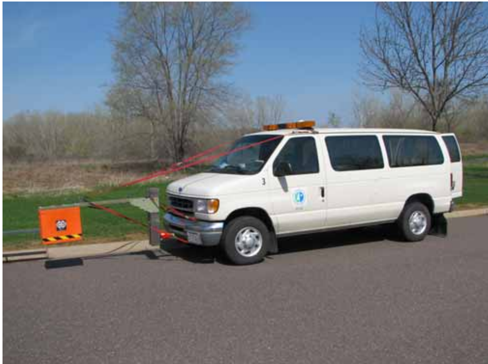
Figure 2.1 Previous GPR vehicle antenna mount
