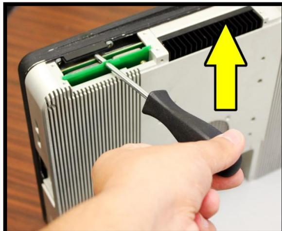
5. To remove the hard drive from the hard drive tray, remove the four screws circled below.
