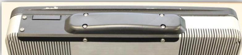
*Cover used when internal antennas are installed.*
