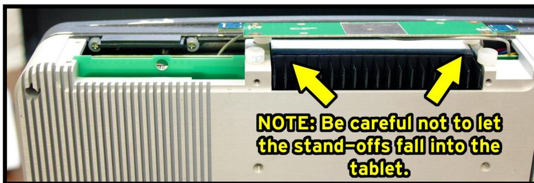
4. While holding the antenna board out of the way, pull out the hard drive tray.
