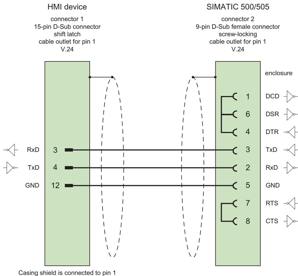
Shield with large-area contact to casing
