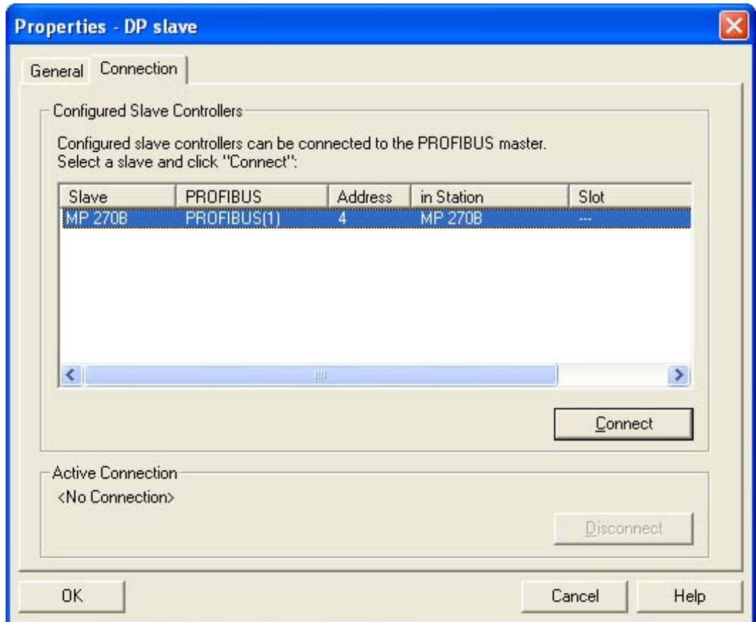
Connecting the HMI device as a slave
