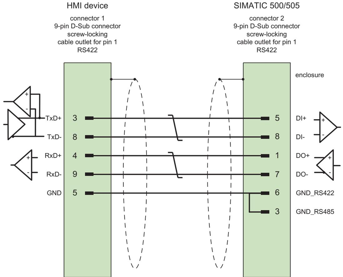
Shield with large-area contact to casing
