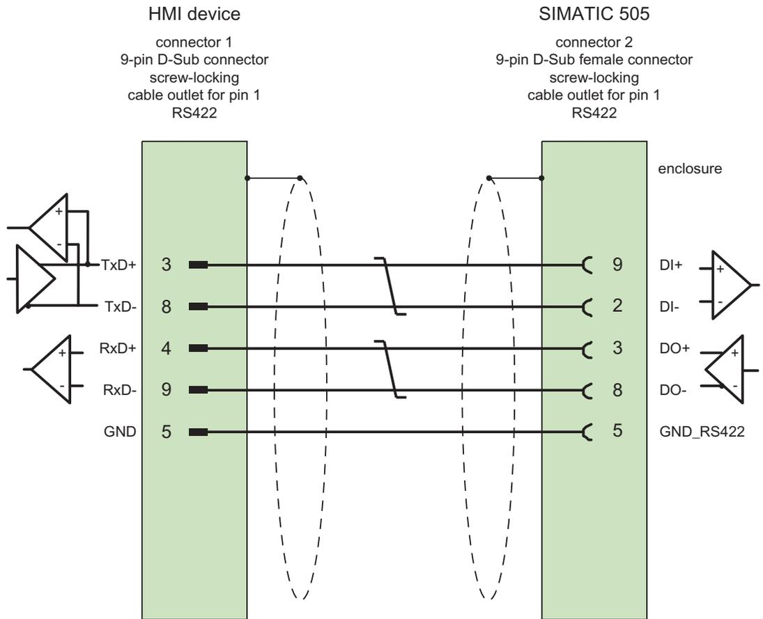
Shield with large-area contact to casing
