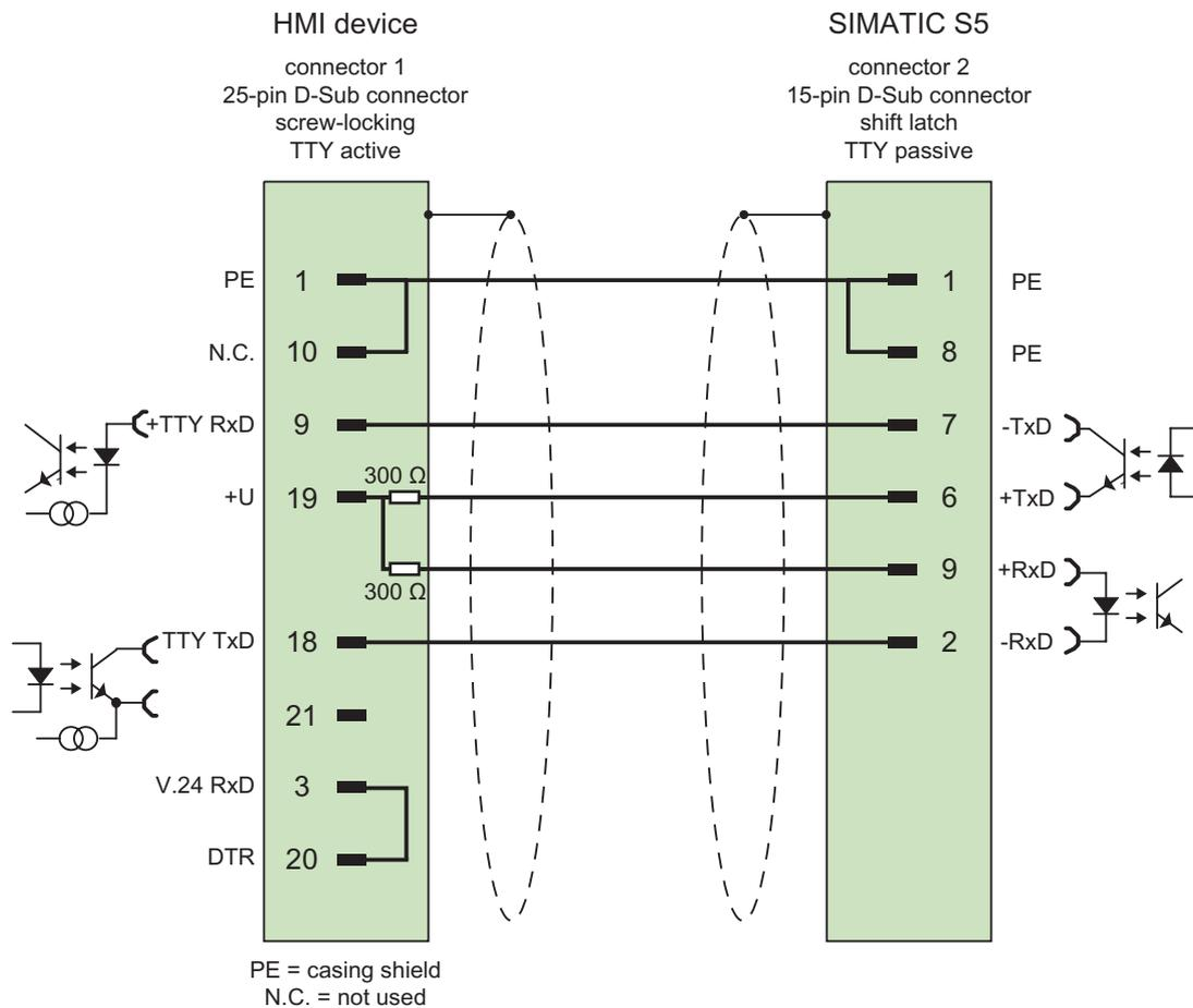
Shield with large-area contact to casing at both ends
