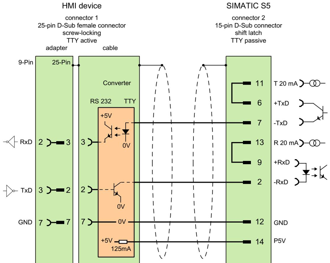
Shield with large-area contact to casing at both ends
