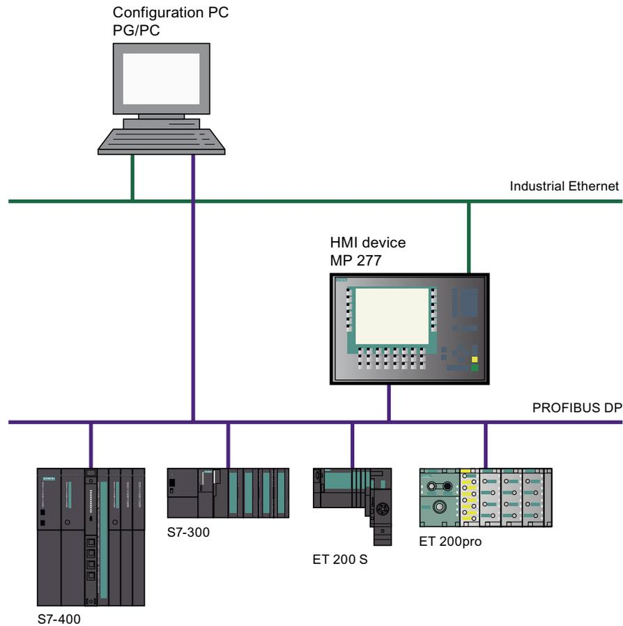
If you wish to control your process using an HMI device and WinAC MP, then you must install WinAC MP on your configuration PC. Then transfer WinAC MP and the project to your HMI device.
