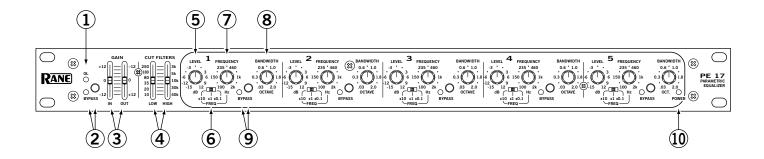
① Overall OverLoad indicator: illuminates whenever the signal level at any of five critical nodes comes within 3 dB of clipping.
