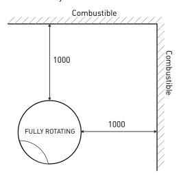
750mm minimum clearance from the back and 1000mm from the side is required if the rotation of the BathyscaFocus Hublot is locked at 90° away from the wall. Locking the BathyscaFocus Hublot so that the opening is fixed is an option available on purchase.
