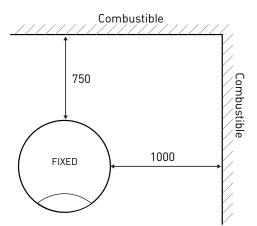
Clearances may be reduced with the application of heat shielding to walls in accordance to the Australian Building Code.
