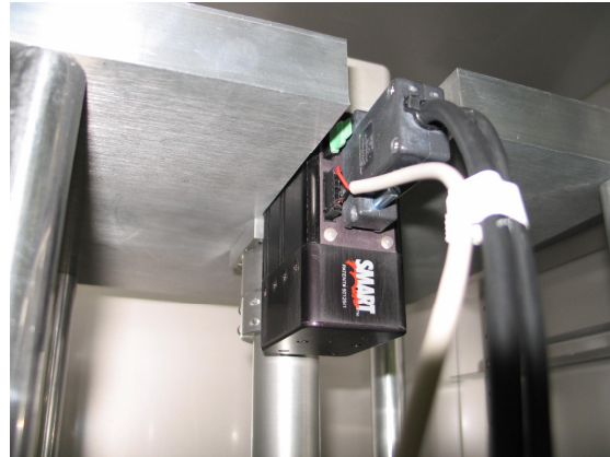
Figure A.2: The amplified load cell signal connection to the SmartMotor actuator (white cable) to input pins.
