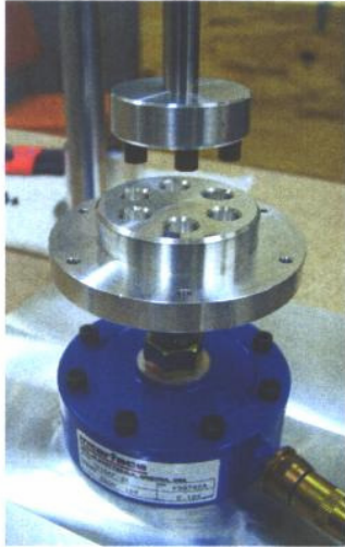
Figure A.1: The dish and load cell assembly of the bioreactor.
