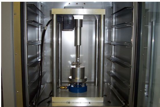
Figure A.3: The bioreactor frame allows the system to fit in an incubator and contains many components that can be sterilized.
