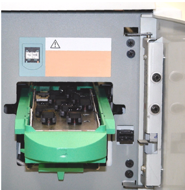
[8] The maintenance cassette
