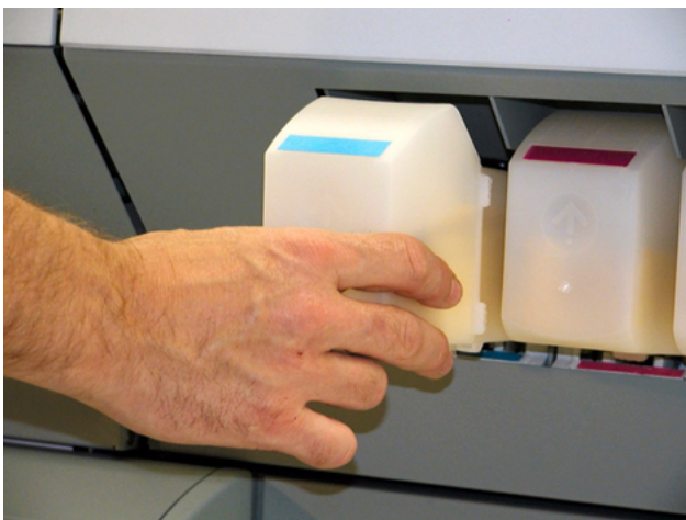
[59] Pull the tank out
