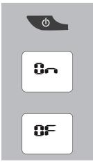
Press and hold the power button for 2 seconds to switch the FR-66 on or off.
