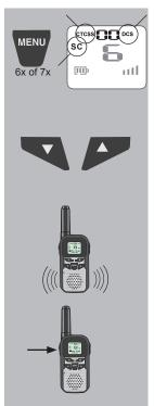
Press 6 x the **MENU** button to start the CTCSS scan or Press 7x the **MENU** button to start the DCS-scan
