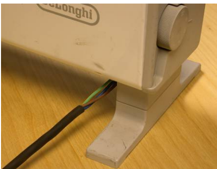
Cable not being gripped.
