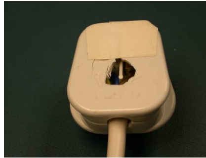
Damage to mains plug.
