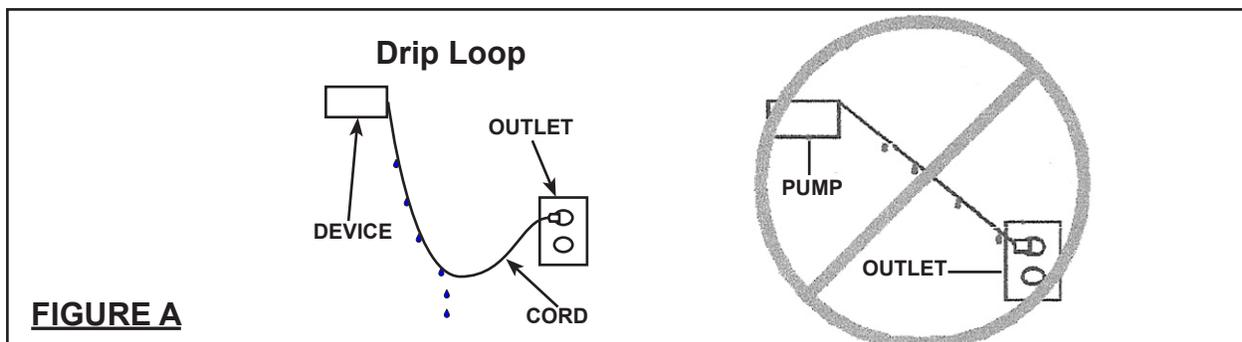
10. ***If necessary***, have a certified electrician install (within 14 feet of where the Pump will be located) a 120 volt, GFCI electrical outlet that is dedicated only to the Pump. Any outlet should be above the water line.
