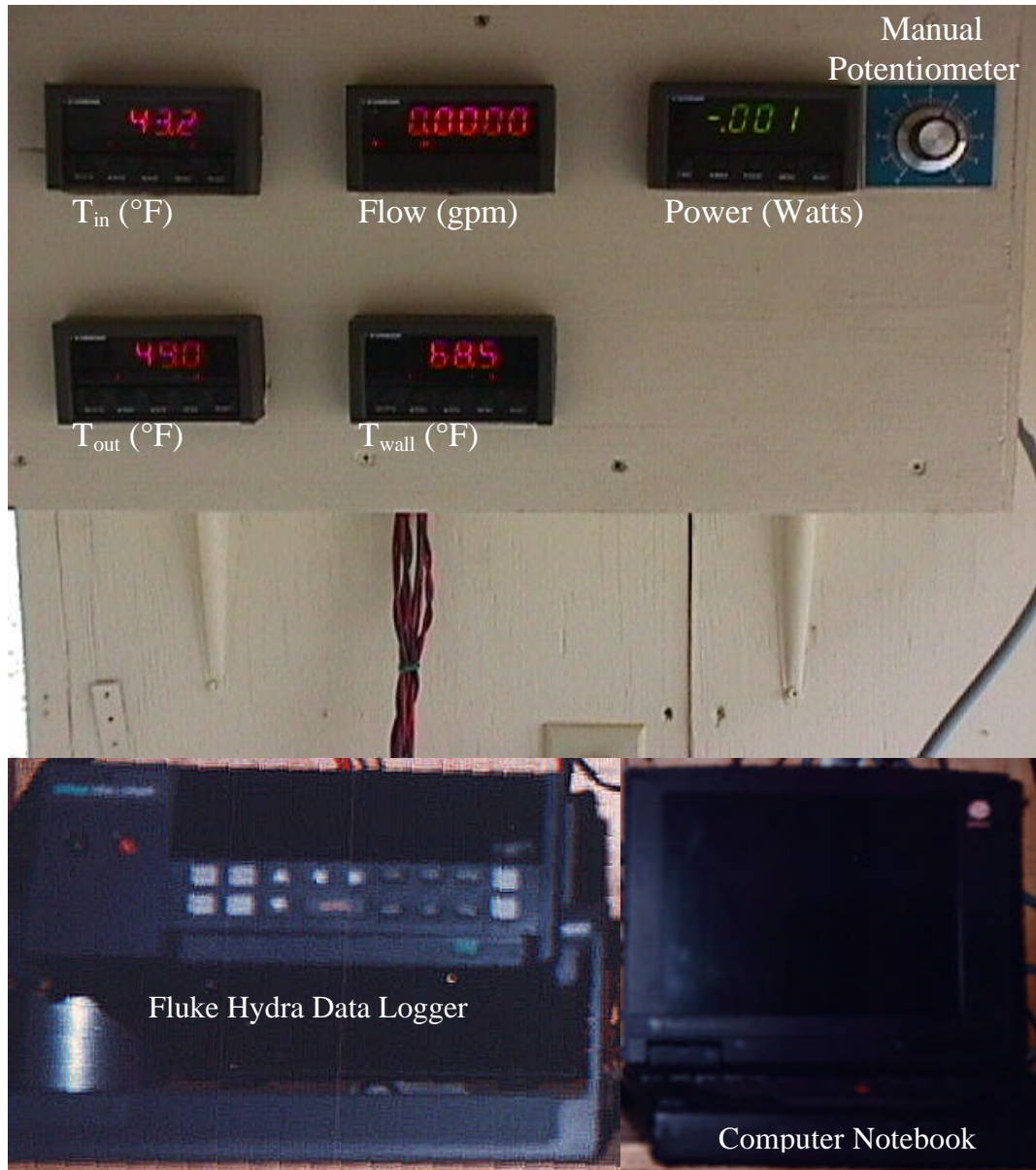
Figure 2-18. Typical Data Acquisition System
