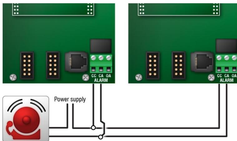
**To connect a normally closed alarm system**
