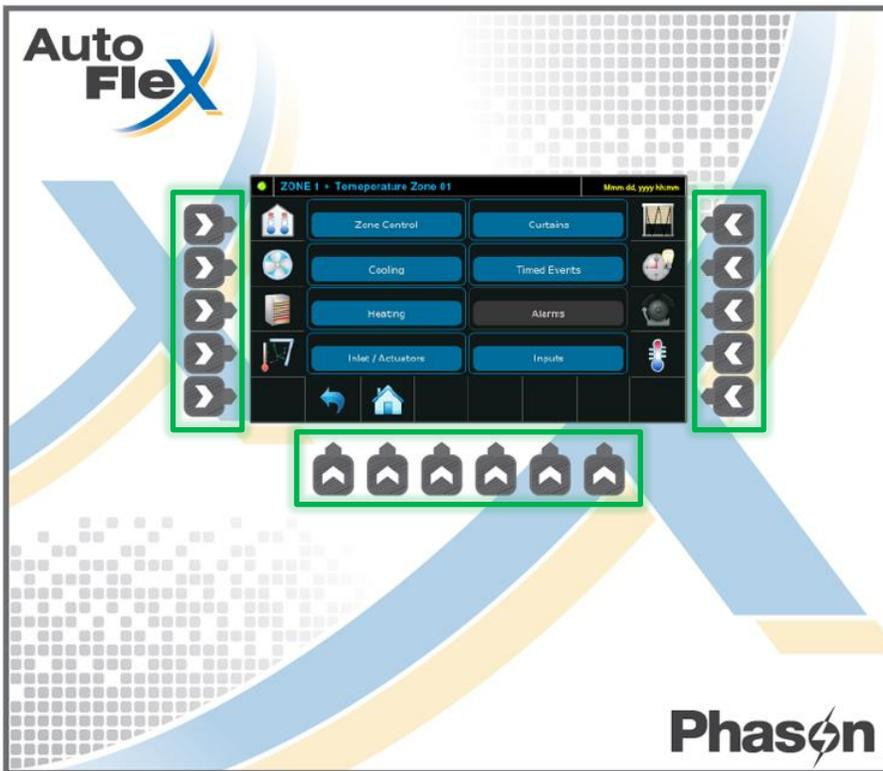
The buttons on the sides and bottom of the display are how you access the control.
