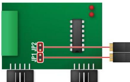
Make sure the shunts are in place for the last device on the communication channel.
