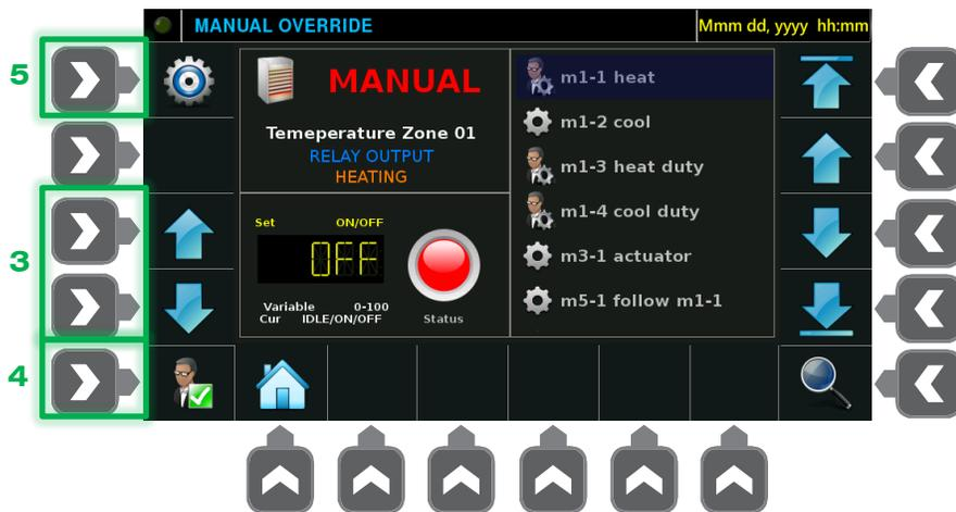
**NOTE** An element stays in manual mode until you put it back into automatic mode or restart the AutoFlex.
