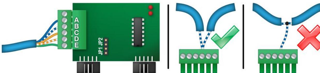
Connect the communication wires to the **ABCDE** positions on the communication connector, **in the order shown**. The order must be the same at each device. When continuing from one device to the next, connect the two wires to each position in the connector; **do not use branches or T-connections**.
