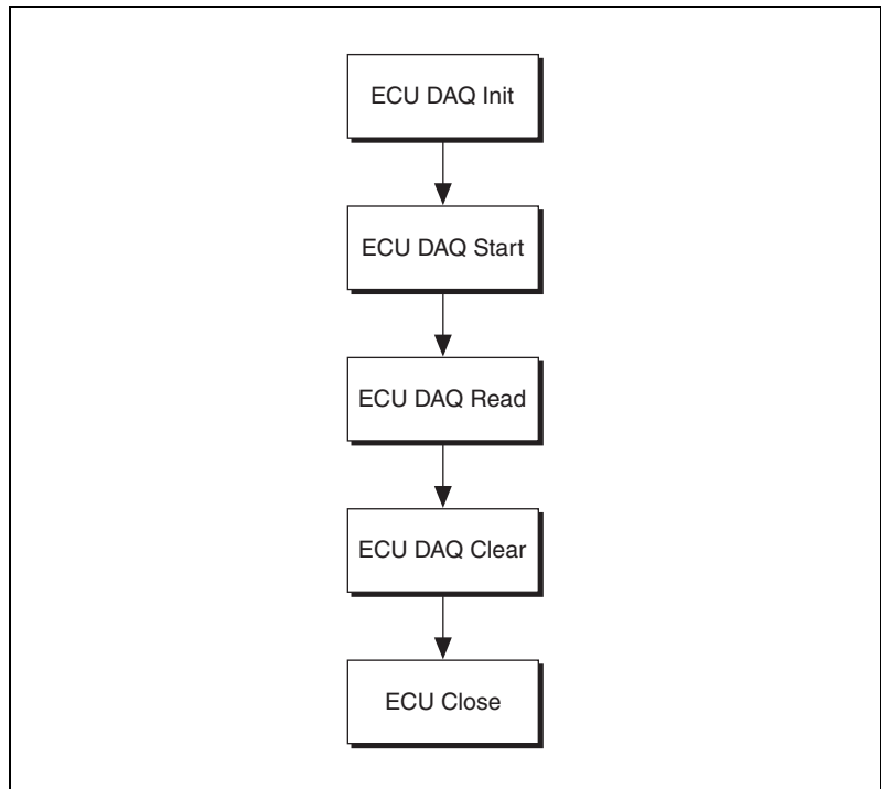
Figure 4-3. ECU Measurement Setup Flowchart
