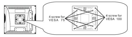
Use only M4 x 12mm screws to mount the VESA bracket, failure to observe this may cause serious injury.
