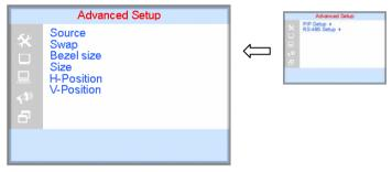
Source: This feature allows a user to select the video input signal to be displayed when in PIP mode.
